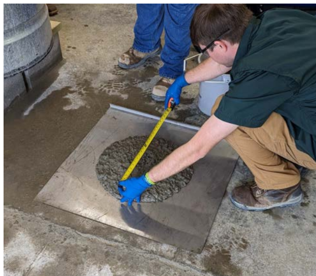
Wet Mix Slump Flow Testing
